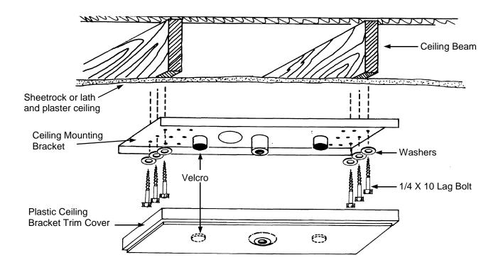
NOTE: THE OUTER ROW OF HOLES ARE 16" BETWEEN CENTERS WHICH IS THE MOST COMMON BEAM SPACING IN RESIDENTIAL WOOD FRAME CONSTRUCTION.
